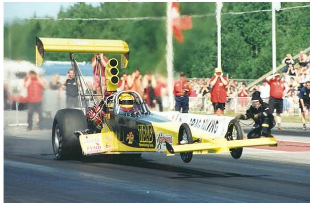
The PLR dragster was equipped with a revolutionary injector hat known as the Sharkfin, which was designed by Morgan. The injector sat in clean air high above the roll cage and blower pulley. The blower design was also changed to front-load the air pressure since at that time 90% of the air went towards the back of the blower. Now standard practice worldwide, the idea was way ahead of its time in the 1990s.
