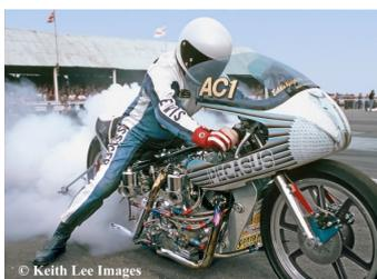
In 1974, Derek and Ian unveiled the double-engined 1656cc Pegasus Norton - a true work of art. Early times were fraught due to an overworked motorcycle gearbox and clutch. Once the bike was fitted with a Lenco two speed and slipper clutch, the wins started coming again. Eddie Keightley joined them as a team crewman.
